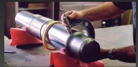
After disassembly, all parts are inspected for wear to determine replacement needs.
